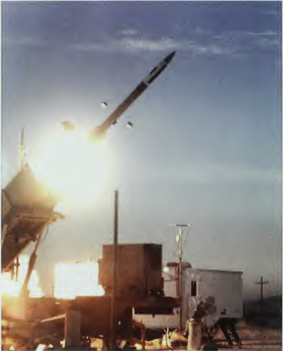
Fig. 5-13. The PAC-3 uses an attitude control system made of a ring of small solid rocket thrusters which provide “the extremely rapid air frame response accuracy to achieve hit-to-kill performance.” Compared to its predecessor, the PAC-2, the PAC-3 can protect an area seven times greater and is effective against chemical and biological warheads. Photograph taken on 5 February 2000.
